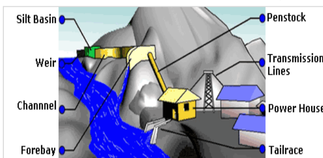
Figure 1. The schematic diagram of an MMHP
