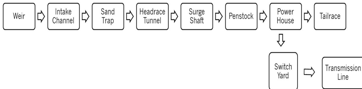
**Figure 3.1: A schematic drawing of proposed project facilities**
